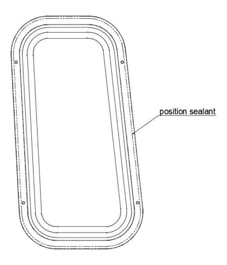
Figuur 3 Application position sealant
